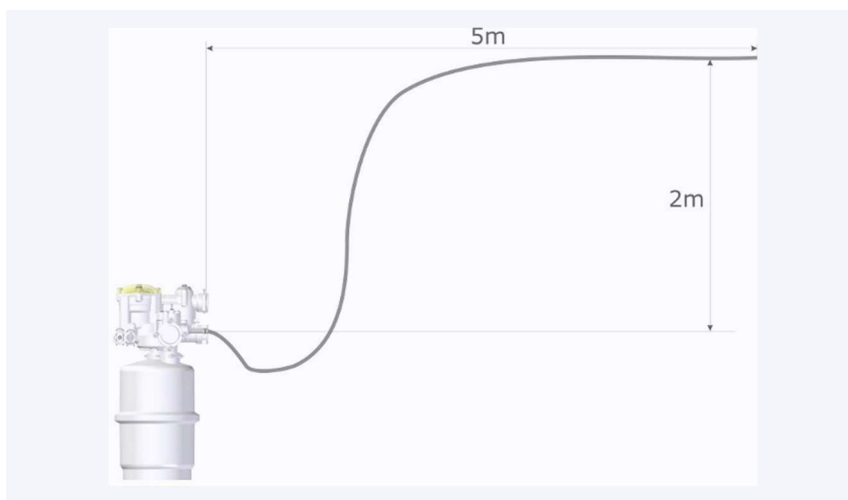
Maximum height and distance of flexible drain hose
